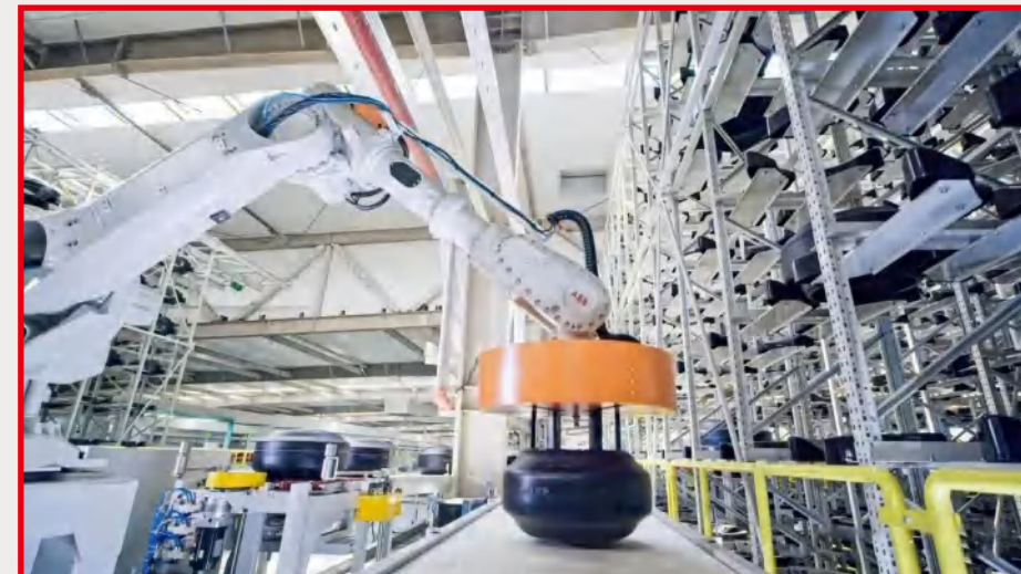
Green tire automatic logistics transportation system
